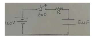
Q4(a) In the circuit shown below, steady state is reached with the switch in position "a". At t=0, switching is done to "b" such that the circuit goes to discharging mode. Obtain the expression for the current i(t).
