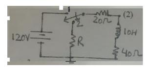
Solution: When the switch is at position 1 for a long time, the inductor acts as short so the final steady state current is  $i(\infty) = V/R = 120/(20+40) = 120/60 = 2A$
